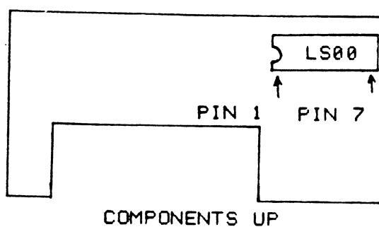
Clip pins 3 and 6 of the LS00 completely off the IC and PC board.
